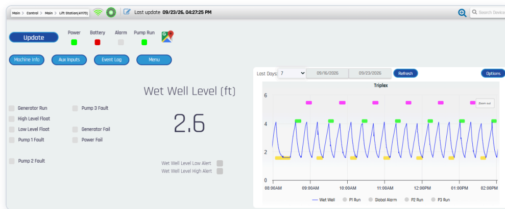
Browser dashboard · wet well level trend with pump run and alarm overlays
